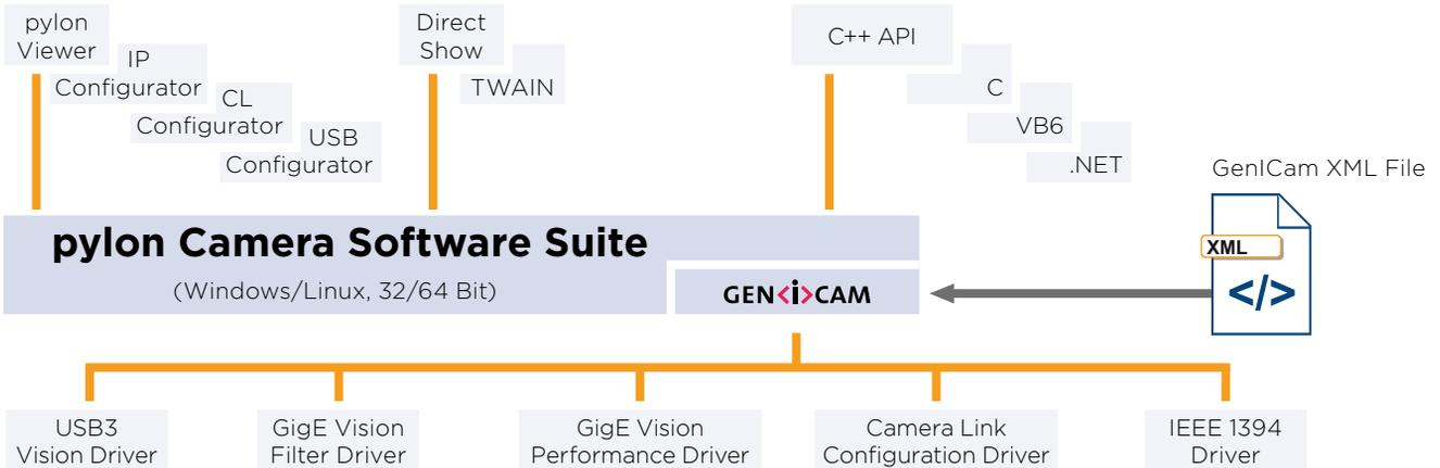
The architecture of the pylon Camera Software Suite is based on GenICam Technology, which offers you easy access to the newest camera models and the latest features. Changes to an existing camera device in your application essentially become a plug-and-play process.
