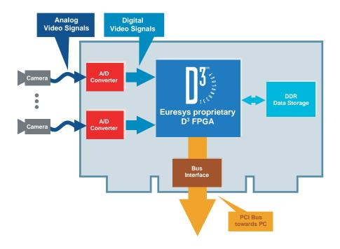
The new Euresys Domino series of analog frame grabbers are based on a proprietary patented technology called D<sup>3</sup> (pronounced D-Cube). D<sup>3</sup> stands for **Digital Domain Decoding**. This innovative technology is applicable to all analog cameras and brings the analog acquisition to its highest quality level.
