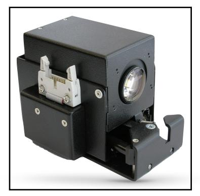
The MPTZ-V2 is a combination of compact pan/tilt and a Sony FCB1000 OEM AF zoom block camera with 36x optical zoom lens.
