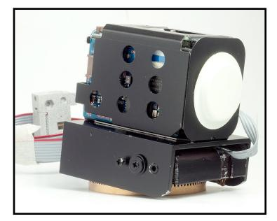
The  $\mu$ PTRZ-20 is a combination of the compact  $\mu$ PTR pan/tilt and a Sony FCB20 OEM AF zoom block camera with 10x optical zoom lens and day/night function.
