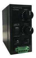
The LC2-PWM20 is a dual channel, pulsewidth modulated LED intensity controller. It outputs 12V PWM from 0-100% at 100kHz to drive LED loads with series limiting resistors. The maximum output is 20W per channel and 30W combined for two channels. Power is limited by the 24V power supply.
