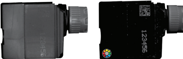
A BP470 Blue Bandpass Filter darkens the background by blocking reflected UV light used to excite the blue fluorescence, creating sufficient contrast.
