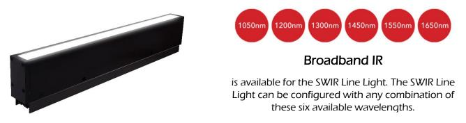
Utilizing a full rod focal lens, the SWIR Line Light provides a tight structured beam of light for up to 12 inches (30.48 cm). The optimal working distance is 5 inches (12.7 cm). High uniformity (±10%) makes the SWIR Line Light ideal for front and back lighting line scan applications.
