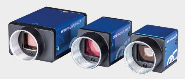
**COE-G series** includes Gigabit Ethernet cameras equipped with the latest sensors, ranging from high speed VGA to the latest 12MP SONY Pregius sensor, which deliver GigE connectivity with high frame rate.
