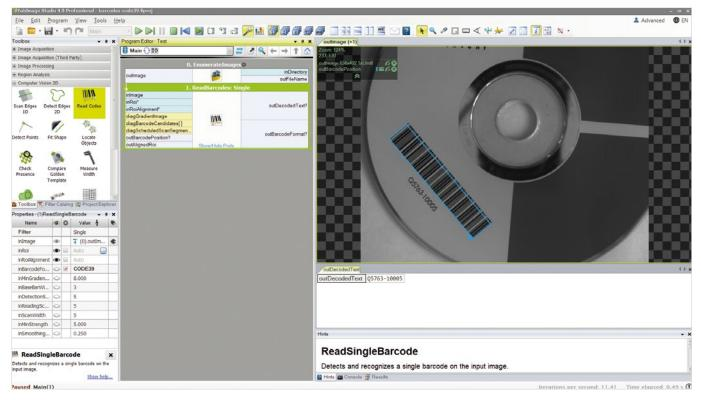
This example shows a basic ReadBarcodes filter. The tool automatically find the barcode and gives as output the decoded text.
