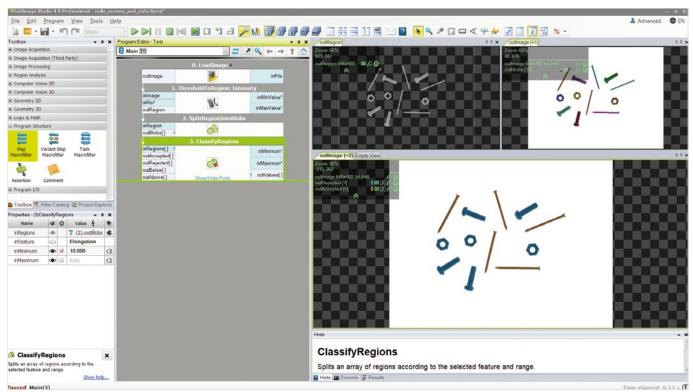
In this application, we need to sort nails amongst nuts and bolts. The image is thresholded and the resulting regions are split into blobs; finally, the blobs are classified by their elongation and the nails are easily found.
