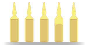
Liquid level inspection.
