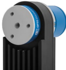
LTPRUP-x models for strobe-only operation featuring ≈ 90W peak power intensity. These models are compatible with CMHO016 clamping mechanics, alternatively three M4 and one M6 threads are available as fixing options.
