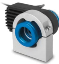
LTPRUP-x models for strobe-only operation featuring ≈ 90W peak power intensity. These models are compatible with CMHO016 clamping mechanics, alternatively three M4 and one M6 threads are available as fixing options.
