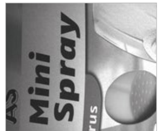
At the Scheimpflug angle, the image becomes sharp.
