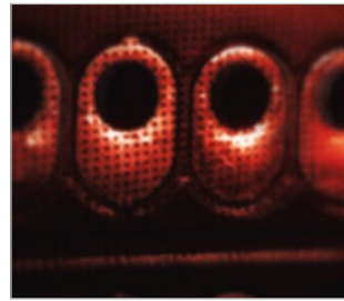
Without tilt adjustment, the image is out of focus.
