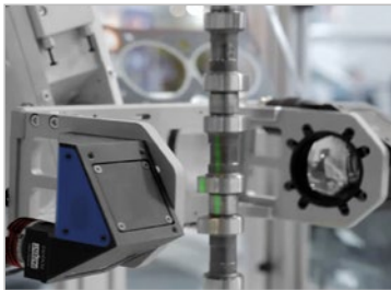
Setup example: 2/3" sensor camera mounted on a bi-telecentric CORE lens TCCR23048, coupled with a LTCLCR048-G telecentric CORE illuminator and a robot holder clamp CMHORBCR048.
