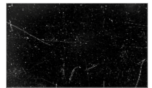
Detection of tiny scratches, bubbles and inclusions on smartphone glass screen.
