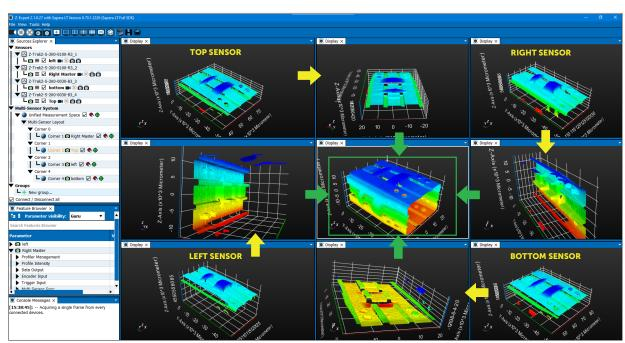
Z-EXPERT 360° View Using 4 Synchronized Z-Trak Sensors
