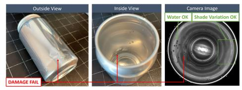
Dents and damage are visible on the inner surface, but natural surface variations and variable water droplets added noise to the image, adding a level of difficulty to the inspection
