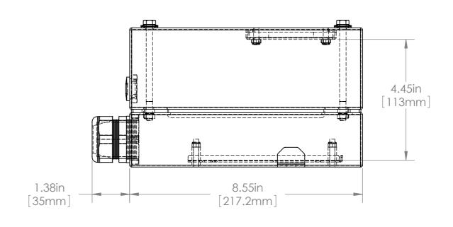
100% 316 STAINLESS STEEL CONSTRUCTION GLASS OR POLY VIEWPORT WINDOW DESIGNED FOR FDA FOOD APPLICATIONS DRILLABLE CORD GRIP W/1.14in (29mm) DIA OPENING 3in (76mm) HEIGHT FOR CAMERA/LENS AIR COOLING/AIR CURTAIN OPTIONS (KIT)
