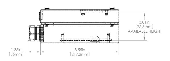
100% 316 STAINLESS STEEL CONSTRUCTION GLASS OR POLY VIEWPORT WINDOW DESIGNED FOR FDA FOOD APPLICATIONS DRILLABLE CORD GRIP W/1.14in (29mm) DIA OPENING 3in (76mm) HEIGHT FOR CAMERA/LENS AIR COOLING/AIR CURTAIN OPTIONS (KIT)
