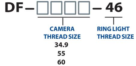
\*When mounting an EZ Mount Ring Light, a double-female adapter is used.
