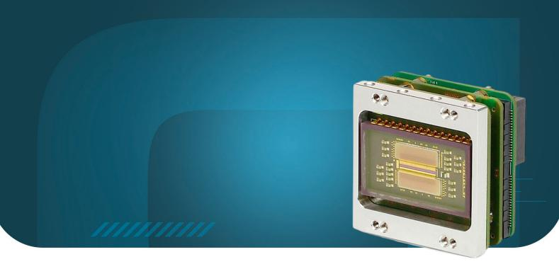
SMALL InGaAs LINE-SCAN MODULE WITH SQUARE PIXELS
